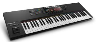
Key lights on your keyboard showing the corresponding colors of the Indie key switches, audio previews and graphical displays. In addition, the rotary controls of your keyboard will be automatically assigned to the most commonly used functions in Indie.
