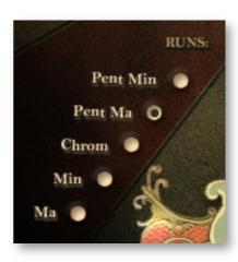
Another neat feature happens when you play a chord and then activate a run. The scripting chooses the furthest played note for a run. With an upward run, the lowest note of the chord will be chosen. Conversely, with a downward run the highest note of the chord will be chosen.
